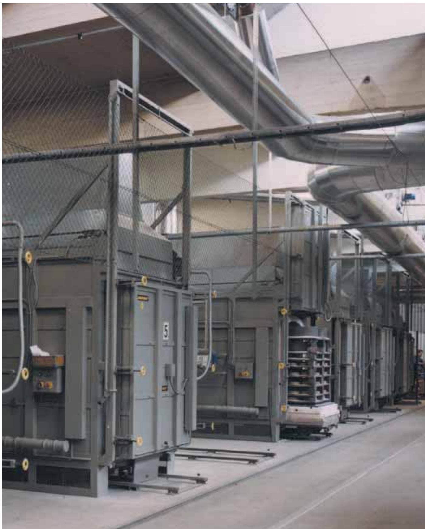
Production line with W 10800/HS1 for sintering grinding wheels
