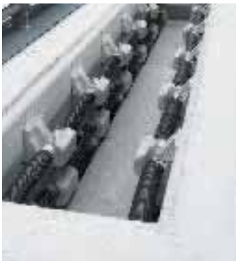
Kiln chamber of the GR 1300/13 with six adjacent chambers
