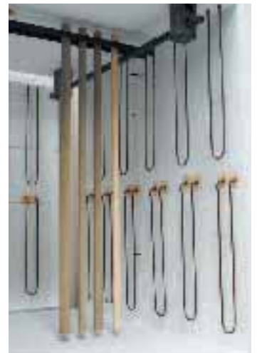
Suspended with ceramic tubes
