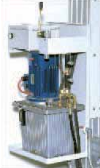
Electro-hydraulic hood drive as standard
