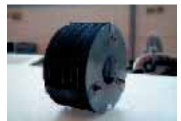
Radiation shield package for reducing the temperature gradient in the working tube
