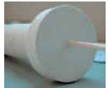
Fibre plug with protective gas connection
