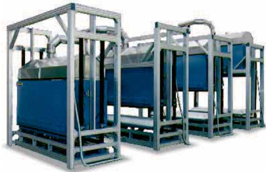
Integrated production system consisting of 4 HT 1010/17 LT furnaces equipped with integrated catalytic afterburner systems for debinding and sintering spark plugs
