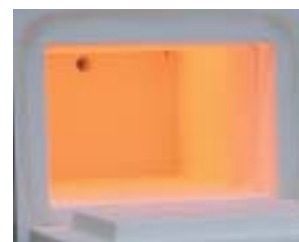
ceramic retort with heating on all sides
