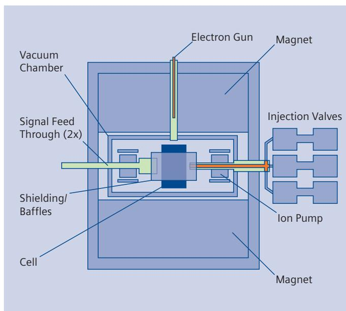
Figure 11: Schematic of the measuring chamber
