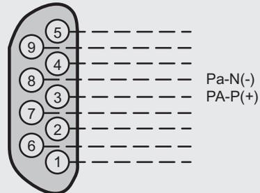
ULTRAMAT 6, 19" unit, pin assignment of Autocal board and PROFIBUS connectors
