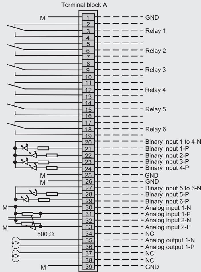
Contact loading max. 24 V/1 A, AC/DC; relay contacts shown: de-energized relay coil
