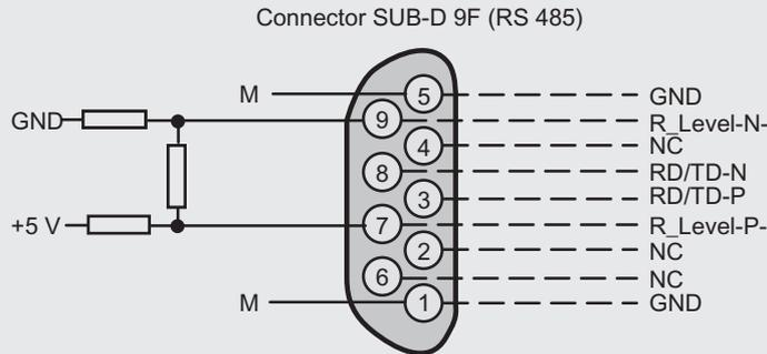
Possibility for connection of bus terminating resistors to pins 7 and 9.
