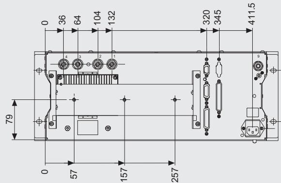
ULTRAMAT 6, 19" unit, dimensions in mm
