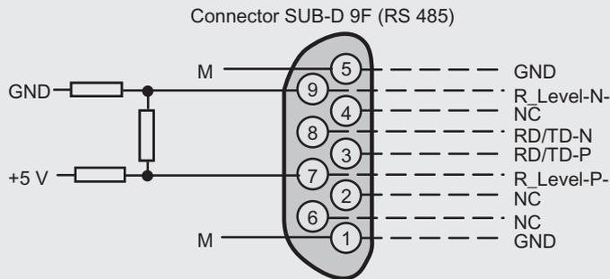
Possibility for connection of bus terminating resistors to pins 7 and 9.
