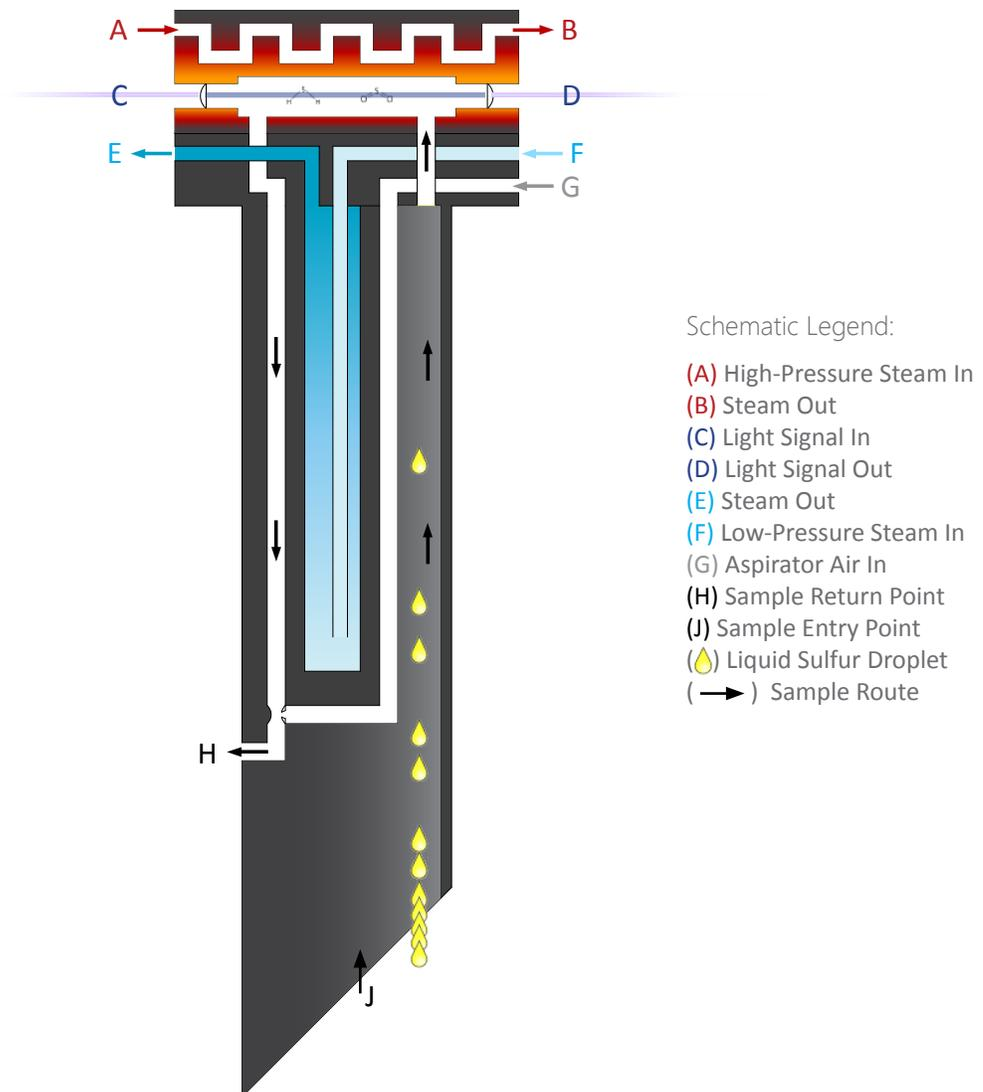
Inside the probe, an internal 'demister' chamber (concentric to the probe body) is fed with low pressure steam (see **E & F**). Since the LP steam is much cooler than the tail gas, this chamber has a cooling effect on the rising sample.
