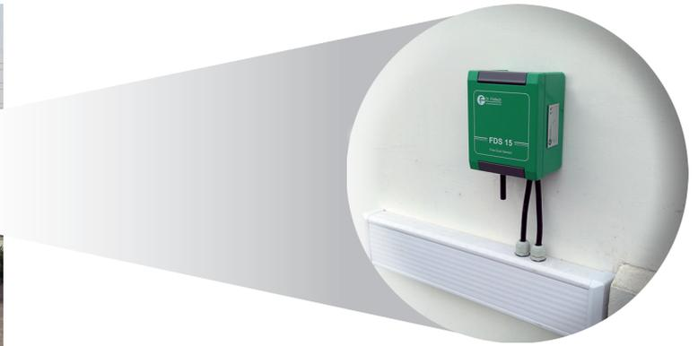
For monitoring the fine dust content at factory premises of the company SNF Floerger a FDS 15 has been mounted at the outer wall of an office building. By means of this outside installation the own production shall be controlled as well as the actual fine dust content of the ambience shall be monitored.
