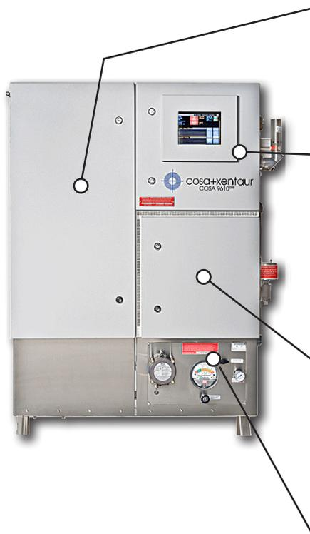
The **gas mixing compartment** contains sample conditioning and the gas mixing system. Components in this compartment are intrinsically safe. The gas mixing compartment can optionally be heated to avoid condensation of heavier gas constituents.
