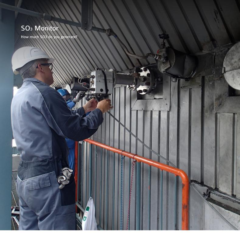
Sulphur trioxide (SO<sub>3</sub>) is formed as a by-product during the combustion of fossil fuels for power generation and is also used or produced in many industrial processes. At temperatures below about 200 °C, it combines with water vapour to form sulphuric acid which has deleterious effects on plant surfaces and on the environment.
