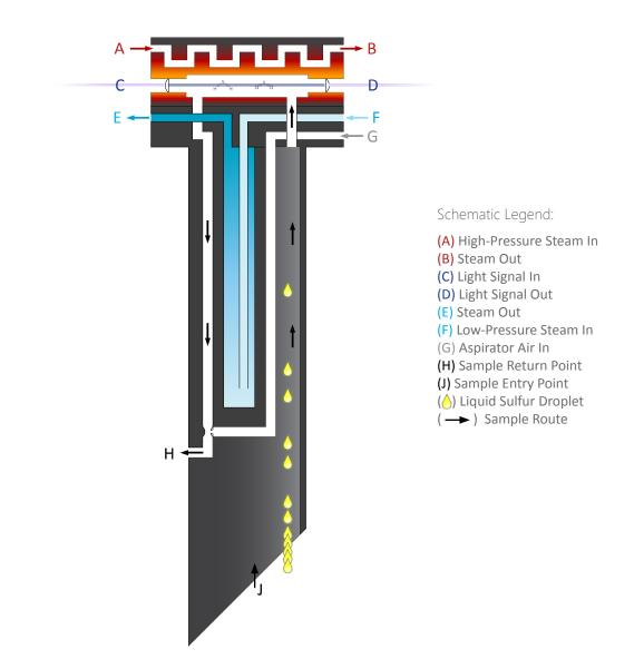
Inside the probe, an internal 'demister' chamber (concentric to the probe body) is fed with low pressure steam (see **E** & **F**). Since the LP steam is much cooler than the tail gas, this chamber has a cooling effect on the rising sample.
