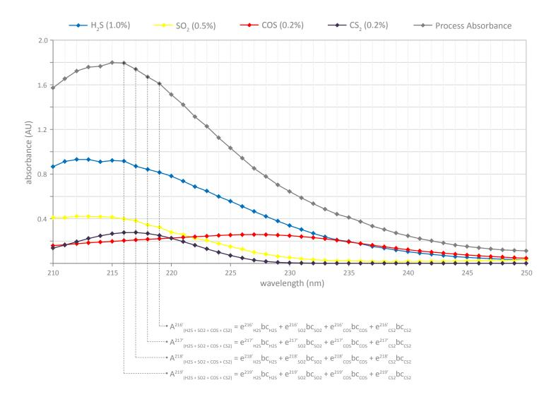
The TLG-837 measures the total absorbance curve of the tail gas and solves for the individual absorbance curves of the analytes by using a matrix of equations. As illustrated above, each photodiode-wavelength combination supplies a single equation to the matrix, in the form:
