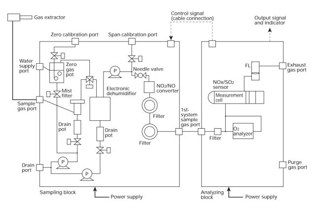
With 2 optical systems (3 to 5 component gas sampling system including NOx analyzer)
