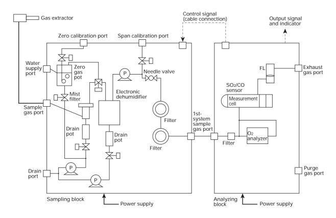
With 1 Optical System (1 to 3 component gas sampling system except for NOx analyzer)
