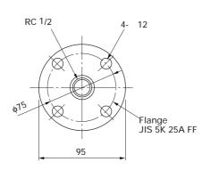
Attached joint (for \u00f66 pipe connection)
