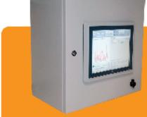
Multi-component, multi-range FTIR gas analyser with embedded touchscreen controller
