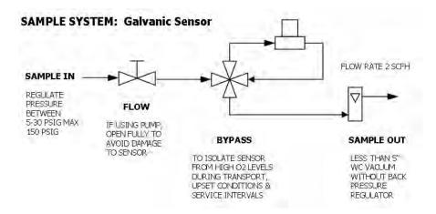
The advantages of the bypass sample system include:
