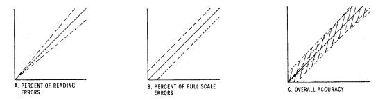
**Example 1:** As illustrated by Graph A any error, play in the multi-turn span pot or the temperature compensation circuit, during a span adjustment at 20.9% (air) of full scale range would be multiplied by a factor of 4.78 (100/20.9) if used for measurements of 95-100% oxygen concentrations. Conversely, an error during a span adjustment at 100% of full scale range is reduced proportionately for measurements of lower oxygen concentrations.
