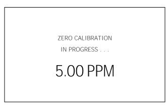
After the oxygen reading has stabilized, press ENTER to complete the Zero Calibration. If the user attempts to initiate the ZERO CALIBRATION function while the oxygen reading is above 50% of the most sensitive or lowest range, the system displays the message "CALIBRATION FAILED" and returns to the "Sample" mode.
