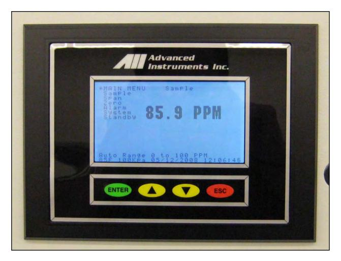
Note: In the event power to the analyzer is interrupted, the system defaults to the "Standby" mode when power is restored. To resume sampling, advance the cursor (\*) to "Sample" mode, press ENTER to select and select the range mode as described below.
