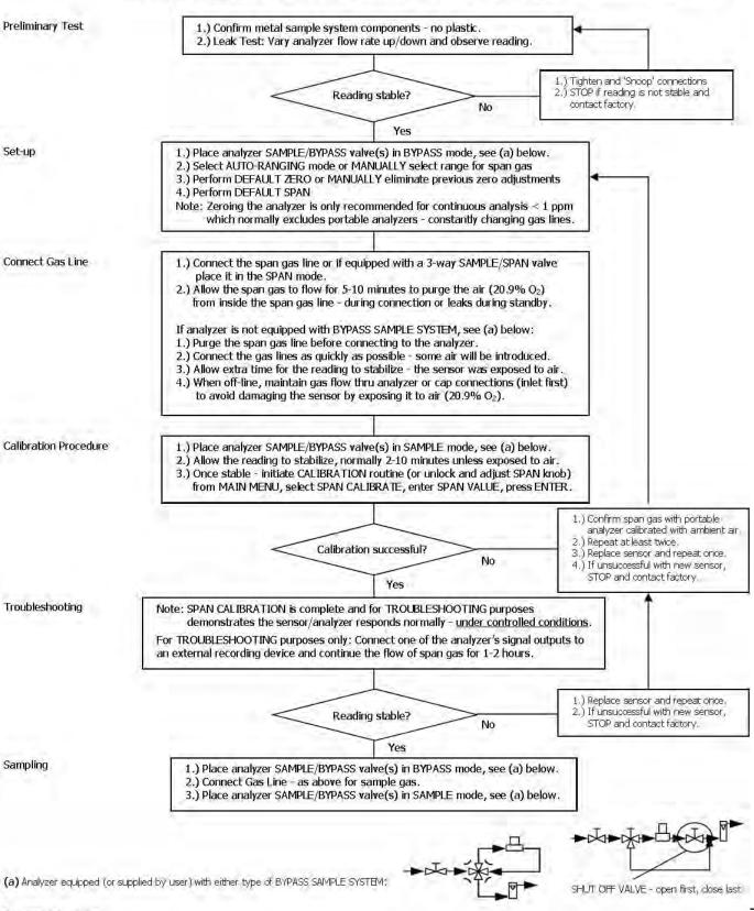
Purpose: AIR CALIBRATION of digital (reference to analog) ppm O2 analyzer (only use for 0-25% range):
