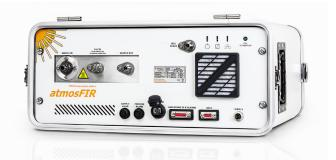
Multi-component, multi-range portable FTIR gas analyser
