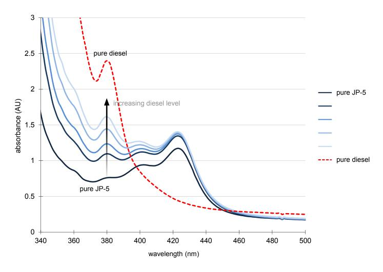
Above, the shades of blue indicate the purity level of the JP-5 sample: lighter blue indicates higher diesel concentration, while the darkest blue indicates pure JP-5. The dashed red curve represents the absorbance of pure diesel.
