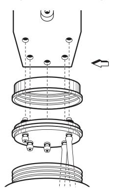
Figure II-7 Reagent Bottle Assembly
