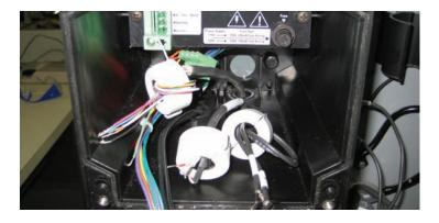
Figure II-8 Ferrite Installation
