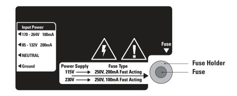
**Note:** Replace the fuse only with a fuse of same rating.
