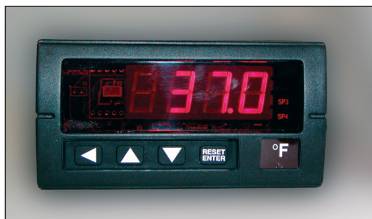
Digital display panel meter provides power and display; relays are optional
