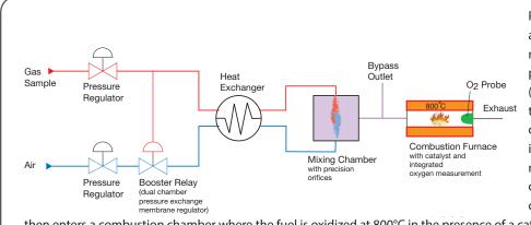
Pressure and temperature of gas sample and instrument air are equalized by means of pre-regulators, a dual chamber pressure exchange membrane regulator (booster relays) and a heat exchanger. The two streams then pass through precision orifices operating at super-critical stage into a mixing chamber. Orifice sizes in the mixing chamber, which are selected based on desired BTU range, precisely maintain a constant fuel-air ratio. The air-gas mixture
