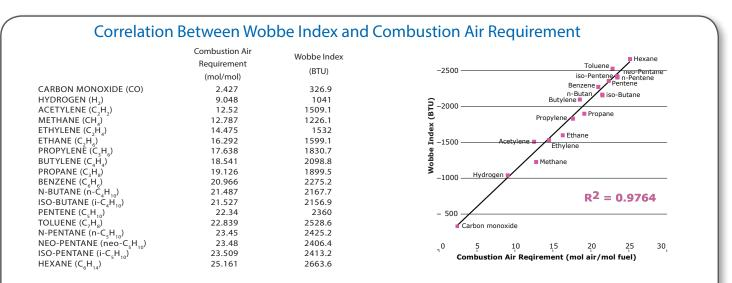
The table and graph above show the relationship of Wobbe Index and the Stochiometric Dry Air Requirement for some typical gas constituents. The correlation is close to linear ( $R^2$ =0.9767) with an intercept close to zero. The residual oxygen method takes advantage of this correlation by linear extrapolation between measurements of known calibration gases.  $R^2$  for typical natural gas constituents plus hydrogen and CO is 0.9888.
